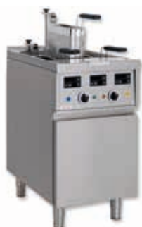
Electric pasta boiler GN 2/3-200 with automatic basket lift for 3 baskets, each controlled separately
