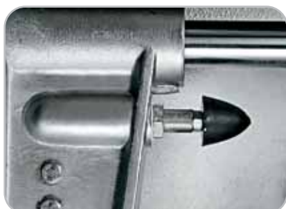
Paracolpo carrello Hopper's buffer
